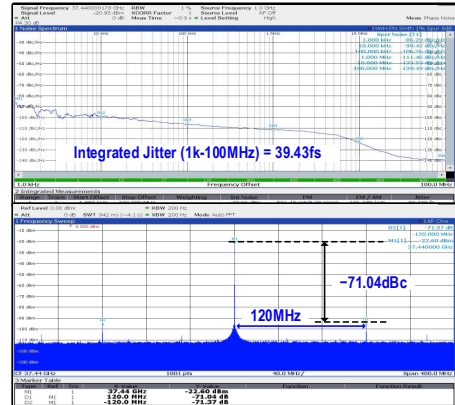
Fig. 7. Measured phase noise and spectra at integer-N channel (37.44GHz).
