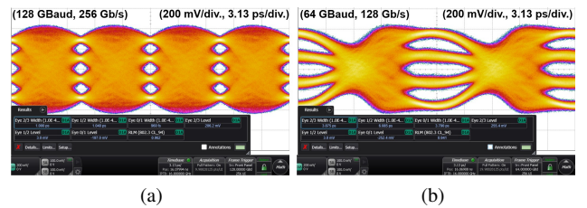
Fig. 12. Measured eye diagrams for a) PAM-4 128-GBaud input passed through the circuit without sampling and b) the demultiplexed PAM-4 64-GBaud eye diagram at OUT1.
